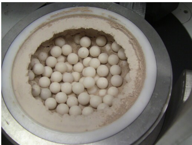
Image 5: Sample 2; caking after a further 5 minutes at 200 rpm
