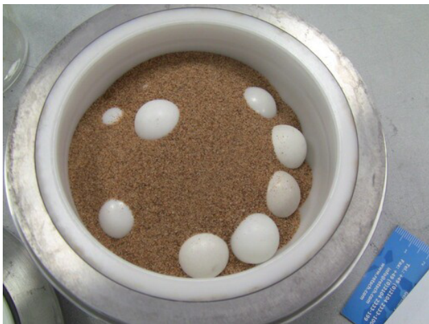
Figure 9: Pre-grinding for wet grinding: 250 ml ZrO 2 grinding beaker + 15 × 20 mm balls
