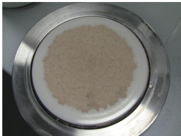
Figure 6: Sample 2; caking after a further 5 minutes at 200 rpm
