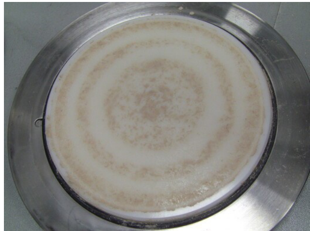
Figure 8: Sample 2; caking after a further 5 minutes at 150 rpm
