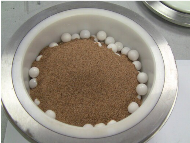
Image 3: Dry grinding: 250 ml ZrO 2 grinding jar + 120 x 10 mm balls
