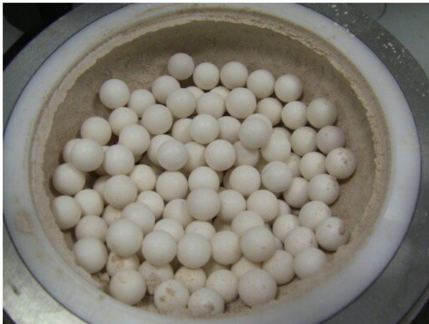
Figure 7: Sample 2; caking after a further 5 minutes at 150 rpm
